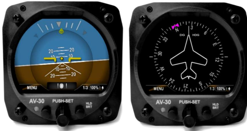
*Figure 1 - AV-30-C Multi Mode AI/DG – Basic Display*
