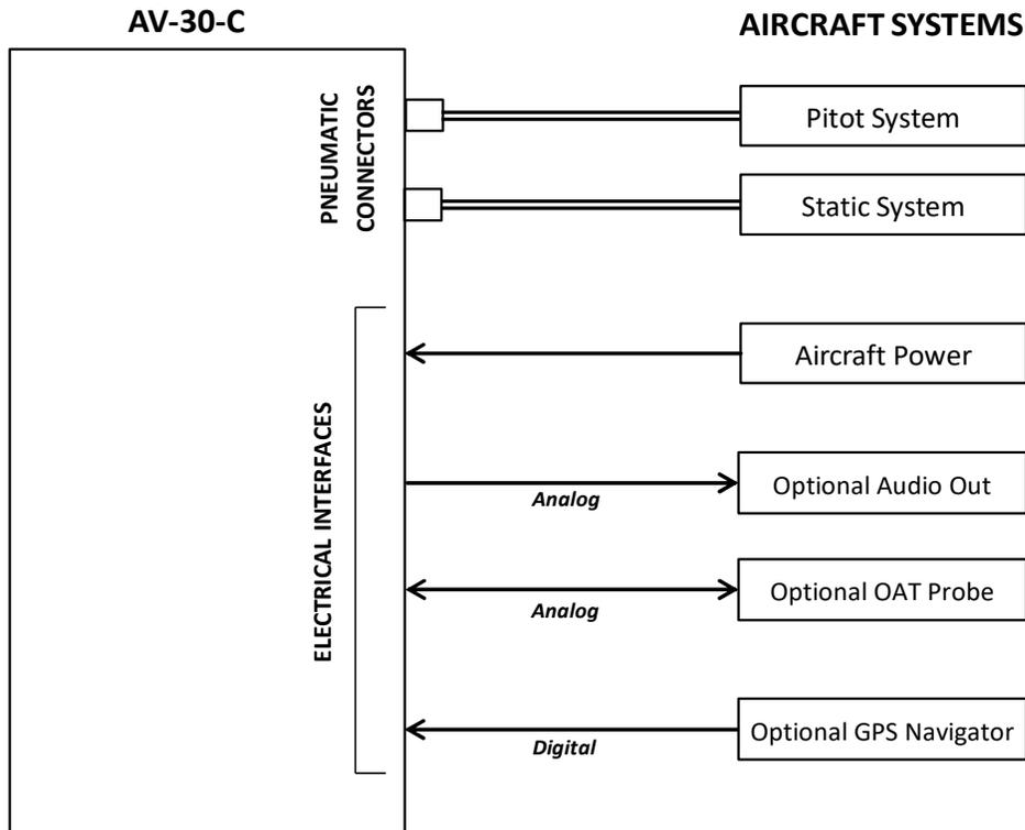
Figure 2 – AV-30-C Aircraft Systems Interfaces – AI Mode
