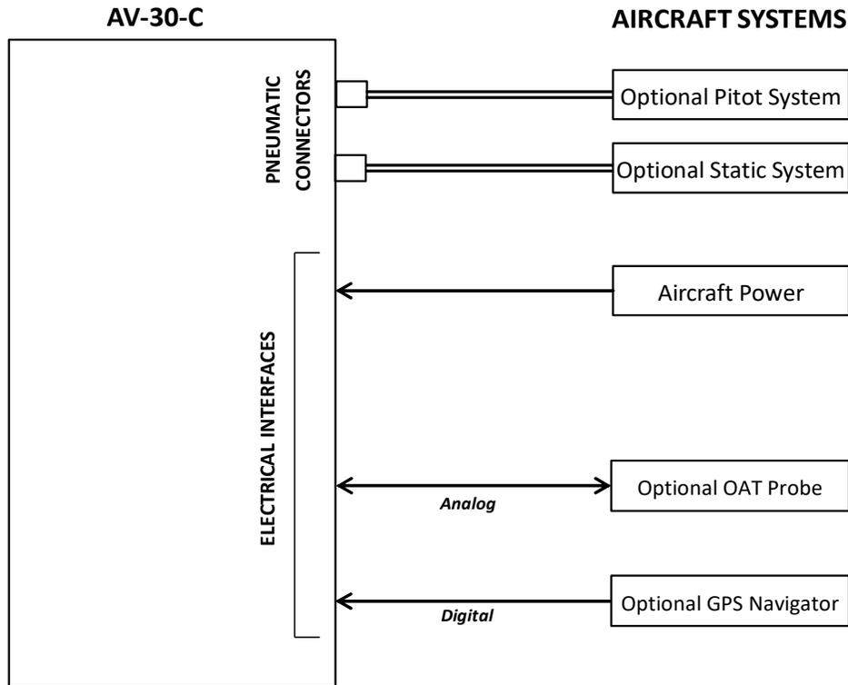
Figure 3 – AV-30-C Aircraft Systems Interfaces – DG Mode
