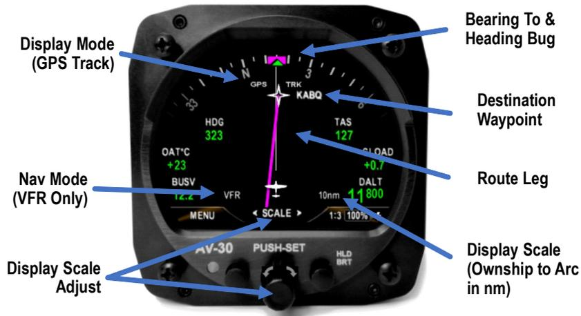
Figure 20 – GPS ARC Mode
